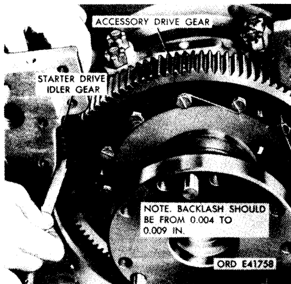
Figure 7-5. Checking accessory drive gear and starter idler gear backlash.
