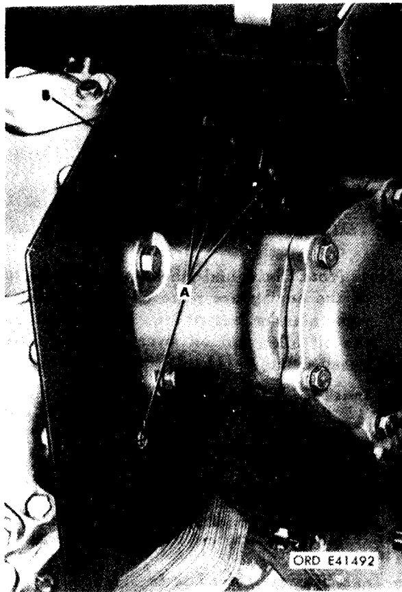
Figure 5-50. Removing or installing right rear shroud.
