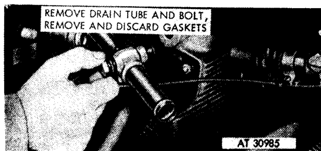
Figure 4-108. Removing or installing intermediate cylinder head oil drain tube-cylinder 2L.
