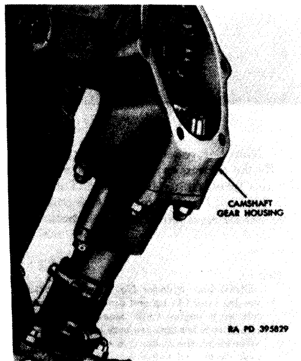
Figure 5-114. Removing camshaft drive shaft using mechanical puller-5120-678-5282.
